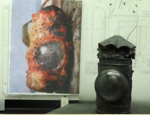
The lantern used on the Confederate submarine H.L. Hunley is seen after conservation in a lab in North Charleston, S.C., on Thursday, April 19, 2012. The picture to the left shows what the lantern looked like after the sub, the first in history to sink an enemy warship, was raised off the South Carolina coast 12 years ago. (AP Photo/Bruce Smith)
